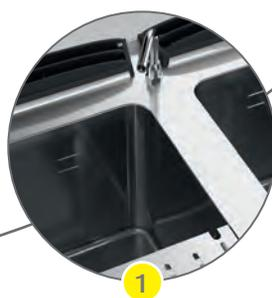
1 PRESSOSTAT DE SÉCURITÉ BLOQUANT L'ALLUMAGE S'IL N'Y A PAS D'EAU DANS LE BAC.
